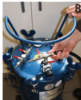
8 Keep the material under pressure for the duration at least equal to its demold time. Then close the air inlet valve.
