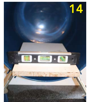
14 Place a wooden board to use as a level surface inside the pressure chamber then follow steps 1 - 11.
