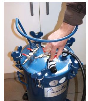
9 Open the air release valves to release the air pressure inside the tank.
