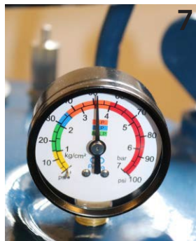
7 While the Pressure tank is rated at >70psi (4.8Bar) it is not recommended to exceed 3.5Bar (50psi)
