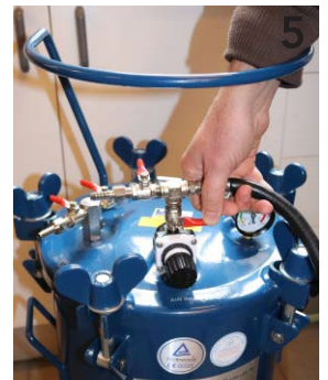
5 Connect your air supply hose. The maximum recommended pressure is 3.5Bar.
