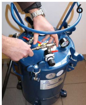
6 Open the inlet valve to release air flow into the pressure chamber.
