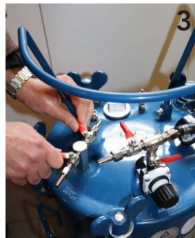
3 Be sure to secure the lid properly by tightening the wing nuts in diagonal fashion for best results.
