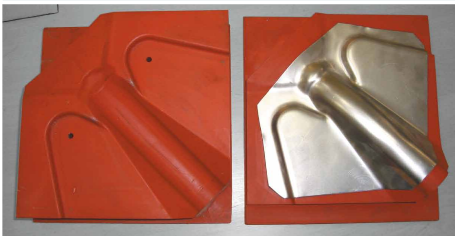
Metal bending tool made from NECURON® 1300
