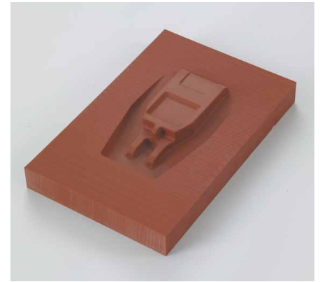
Foundry model made from NECURON® 1300
