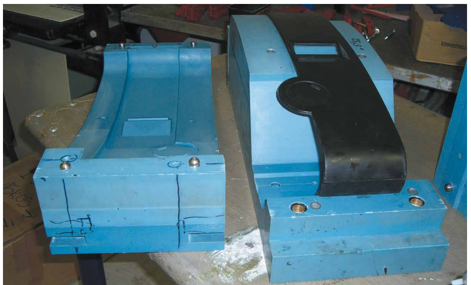
RIM tool made from NECURON® 1020
