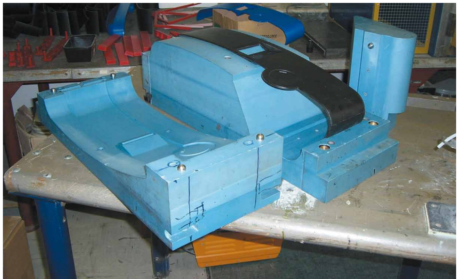
RIM tool made from NECURON® 1020
