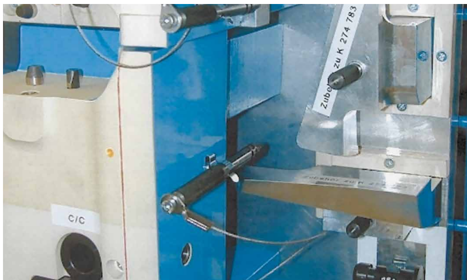
Checking fixture with measuring points made from NECURON® 1007
