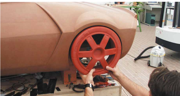
Clay model: substructure NECURON® 100, other parts (wheel and radiator grill) NECURON® 1300
